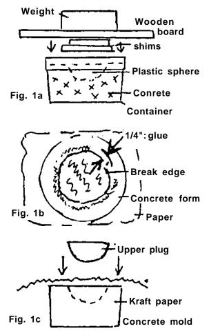
Hint: Applying wax to the sphere halves before placing them in the cement will make them easier to remove from the cured concrete. Automobile wax works fine.
