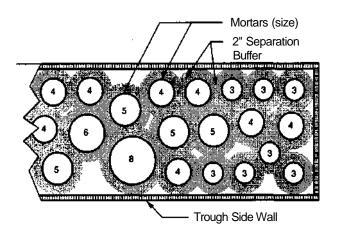
Figure 1. Illustration of mortar placement in a trough using the NFPA two-inch separation. (Overhead view.)
