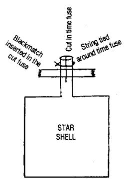
I found that using this method had several advantages, including more accurate timing as to the burn time from the ignition of the shell to the time it would break in the air. This is also a lot easier to do than punching a hole in the time fuse and then trying to insert the blackmatch.
