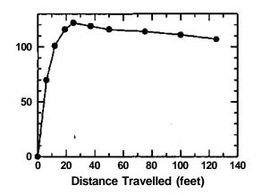
Figure 2. Typical graph of the speed of a Horse Brand sky rocket as a function of distance traveled.
