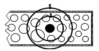
Figure 2. Zones of decreasing blast effect around a mortar explosion.
