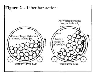
Once the charge is locked to the jar's rotating speed, it can cascade properly. But it cannot grind material unless there is material between the balls when they strike one another. If there is too much material present, it will serve to cushion the blows, and reduce the grinding action. Apparently, there must be an optimum **material charge**.
