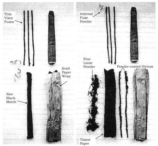
Figure 2. Photos of a dissected shell leader illustrating its construction.
