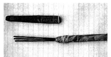
Figure 1. Shell leader containing the new fast burning black match. (Note that the three exposed fuses have been separated slightly for clarity.
