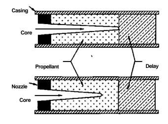
Figure 3. Rocket motors with varying core length.
