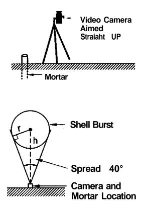
Figure 2. Geometry of a typical hard breaking spherical shell
