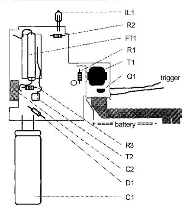
Figure 1 - Drawing of the flash circuit board, component side
