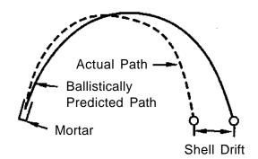
Figure 1. Illustration of drift distance for a dud aerial shell
