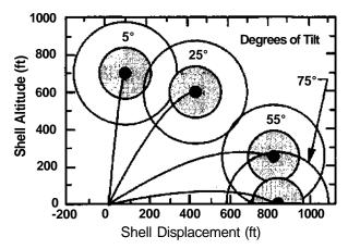
Figure 3. Illustration of the trajectory and functioning of 6-inch aerial shells fired from tilted mortars.
