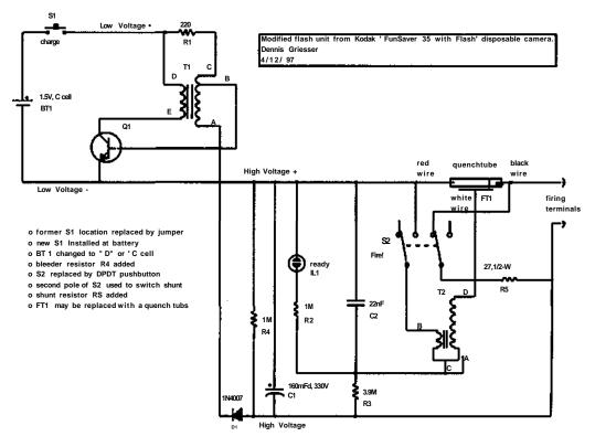
Figure 3 - Tube variation of CD firing box.
