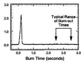
Figure 1. Typical thrust profile of a Horse Brand sky rocket.
