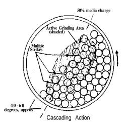
The angle of break will change as the speed of rotation of the jar changes. The slower the rotation, the shallower the slope of the pile. If the jar turns too slowly, balls will simply slide down the sides of the jar, failing to pile up enough to cascade. This causes extremely fast media and jar wear, and is usually manifest by grooving on the inside of the jar, and flat spots developing on the balls. But the jar can spin too fast.
