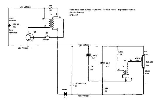
Figure 2 - Flash circuit schematic diagram
